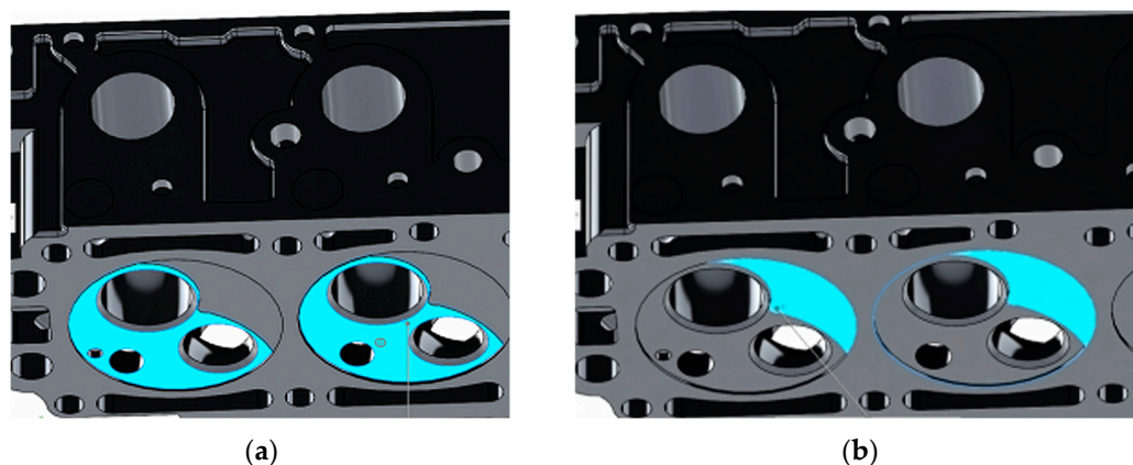
Figure 7. Setting boundary conditions across the combustion chamber surface area: (a) Surface 1; (b) Surface 2.
