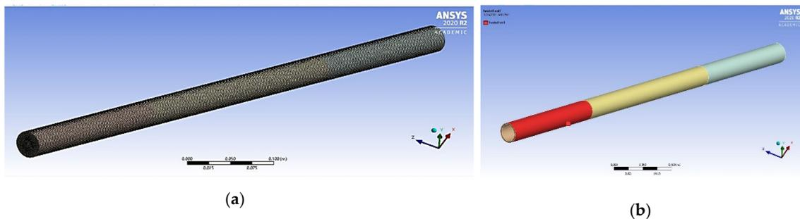
**Figure 1.** (a) Receiver tube meshing. (b) Tube sectioning.
