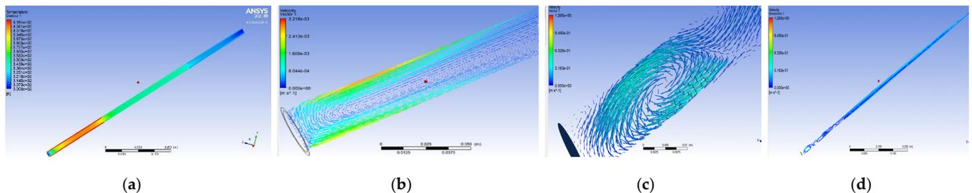
Figure 3. (a) Temperature contours. (b) Velocity vectors. (c) Velocity vectors at heated section. (d) Velocity streamlines.
