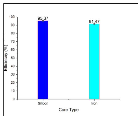
**Figure 4.** Output Core Efficiency (%).
