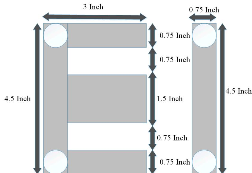
**Figure 3.** EI Core Dimensions.
