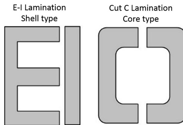
Figure 1. Types of different core laminations.
