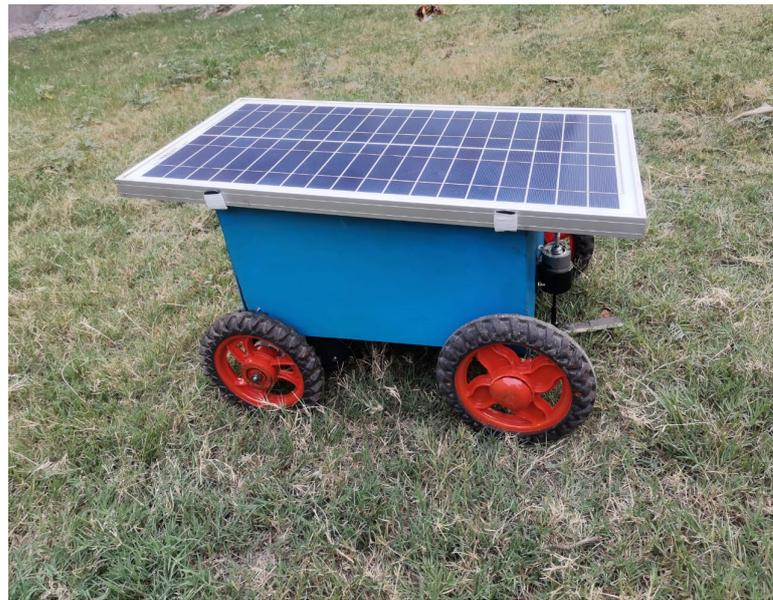
**Figure 1.** Smart solar grass cutter.
