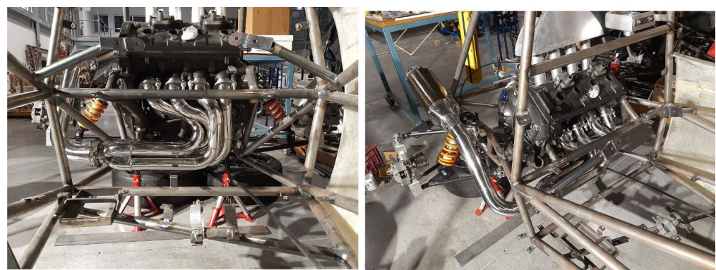
Figure 4. Final assembly of the racing car. Without the intake manifold (Left photo). With the intake manifold (Right photo).
