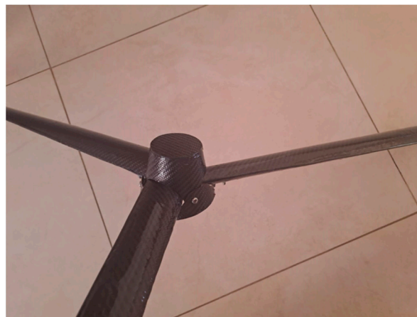
Figure 2. Final fabrication of the blades and the hub of the NREL 5MW scale wind turbine model using composite materials.
