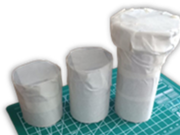
Figure 3. Sample target objects used for dataset generation, from left to right: heights of 5 cm, 7 cm, and 9 cm and cross-sectional areas of 20 cm 2 , 20 cm 2 , and 40 cm 2 , respectively.
