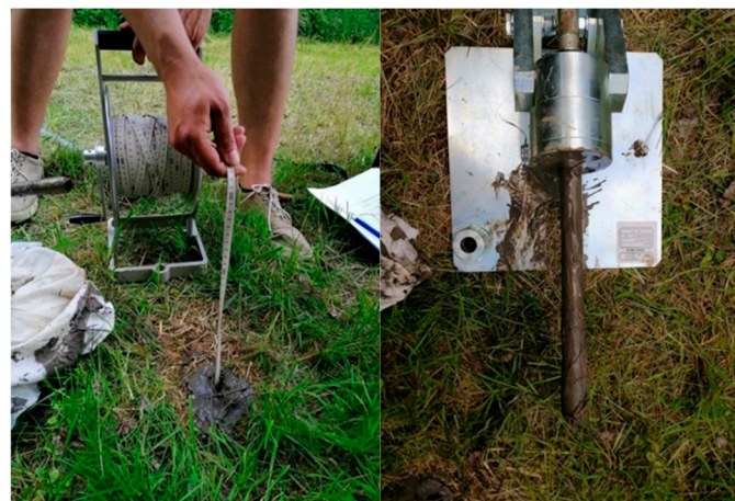
Figure 3. HPV measurement using an electrocontact level meter (left), sample of clay soil in a liquid state on a DPL (right).
