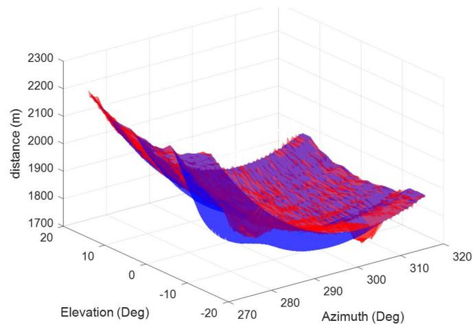
**Figure 3.** Result of surface reconstruction in polar coordinates: raw data (red) and approximated curves (blue).
