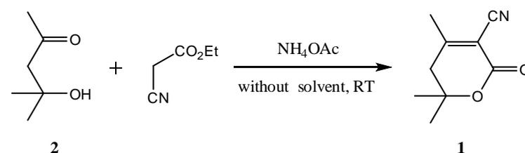
**Figure 1.** Synthesis of 4,6,6-trimethyl-2-oxo-5,6-dihydro-2H-pyran-3-carbonitrile **1**.
