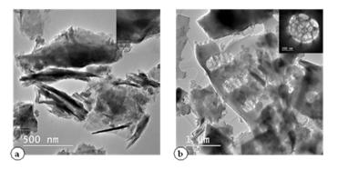
**Figure 1.** Transmission electron microscopy images of activated SNNMs, (**a**) Rupea natural zeolites, (**b**) Pătârlagele diatomaceous earth. From ref. [2]. Copyright: © 2021 by the authors. Licensee MDPI, Basel, Switzerland.
