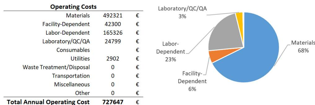
**Figure 6.** Cost components for the simulated operating costs (seed input price/kg = 5 EUR/kg, seed diameter = 6 mm, required coating thickness = 50  $\mu$ m).
