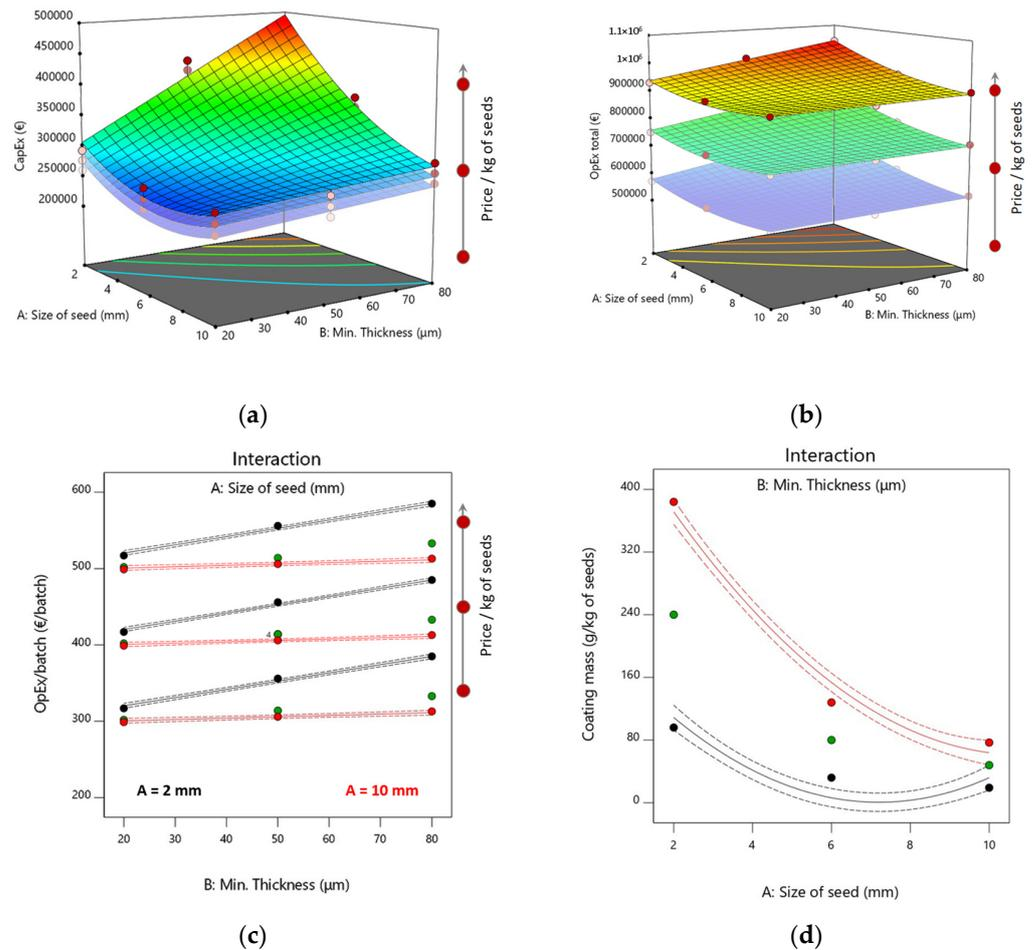
**Figure 3.** (a) The response variables as a function of the input variables: capital costs/CapEx; (b) operation costs; (c) operation costs per package of 50 kg of coated seeds at required thicknesses; (d) coating mass per kg of initial seeds.
