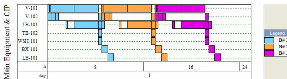
**Figure 2.** Scheduling of the equipment use in a sequence of three batches using SuperPro Designer 10.
