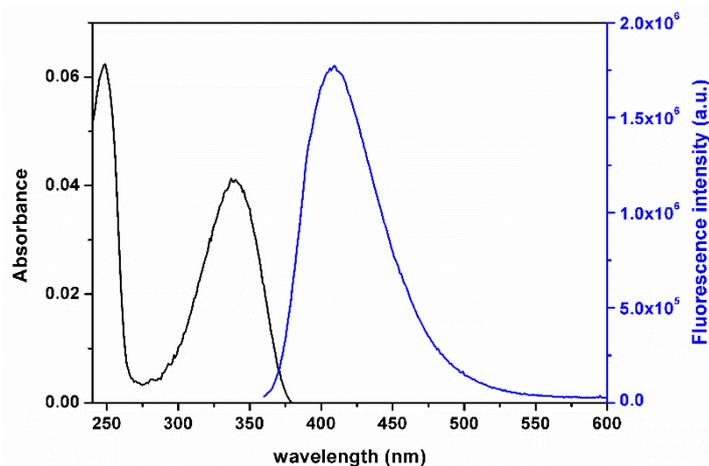
**Figure 2.** Absorption and fluorescence emission (excitation at 340 nm) spectra of compound **3b** in ethanol ( $1 \times 10^{-5}$  M for absorption and  $1 \times 10^{-6}$  M for emission).
