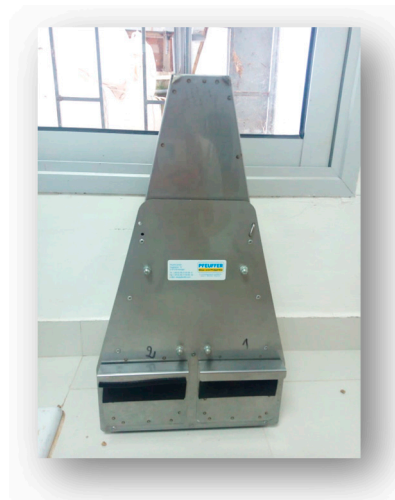
Figure 2. Sample divider used to split bulk samples into representative subsamples.
