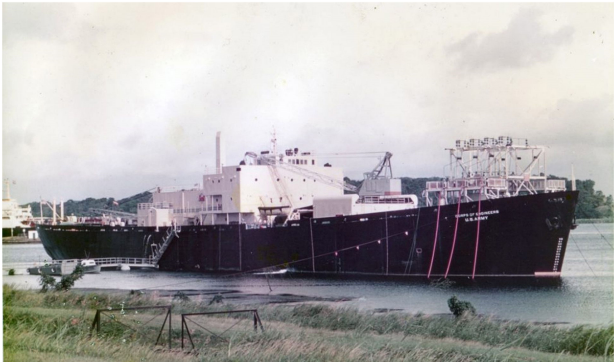
Figure 6. Sturgis , floating nuclear power plant operating in the Panama Canal Zone. The electrical substation is seen on the bow. Photo credit: U.S. Army Corps of Engineers (circa 1970).
