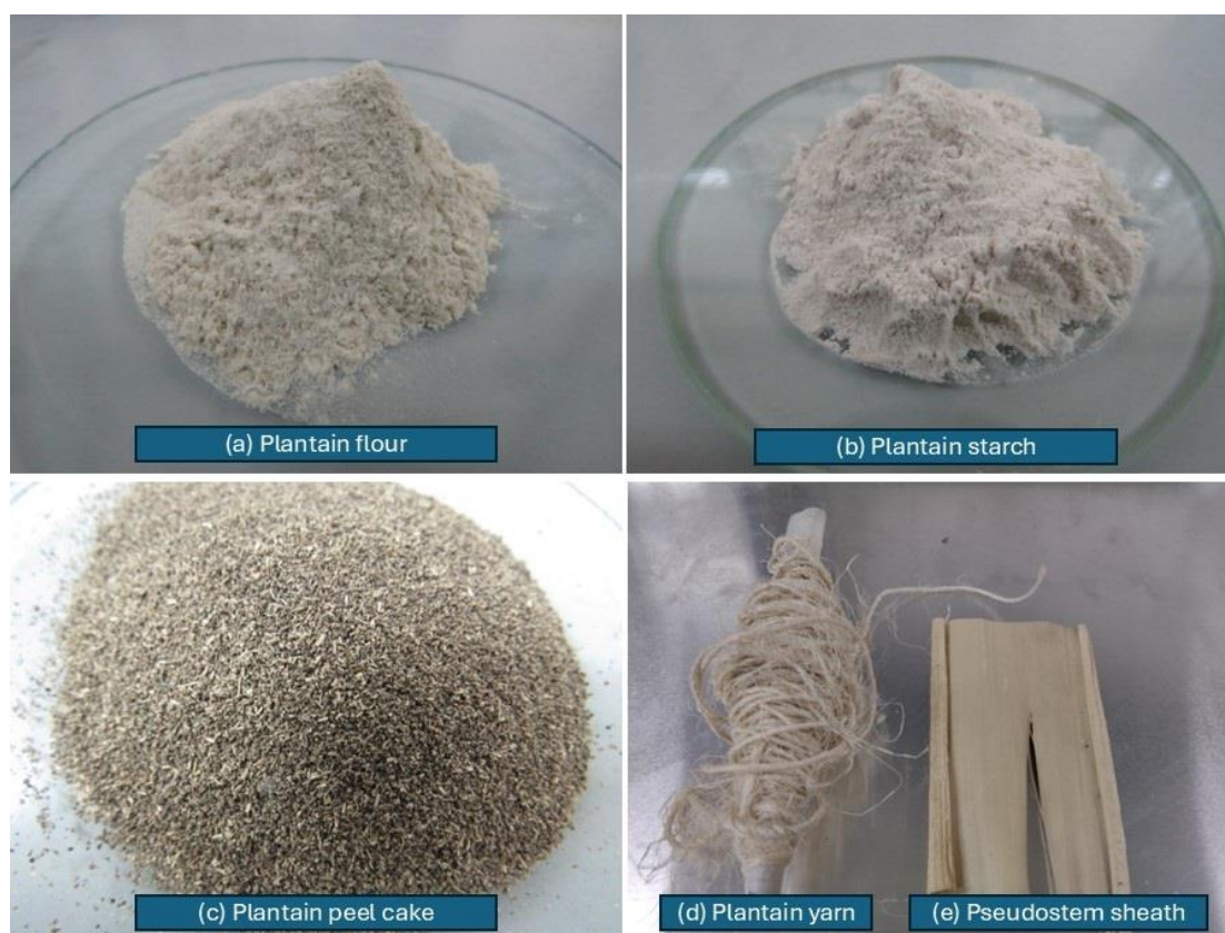
Figure 1. Plantain-based raw materials used for the development of BCMs: (a) plantain flour; (b) plantain starch; (c) plantain peel cake; (d) plantain yarn; (e) pseudostem sheath.
