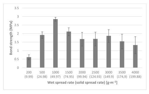
**Figure 3.** Influence of the spread rate on bond strength (10 min of drying time, 55 °C of drying temperature for 105 min) for the CSA adhesive.
