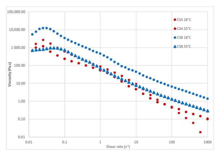
Figure 4. Influence of the shear rate on the rheological curves of the CSA and CSB solutions at 18 °C and 55 °C.
