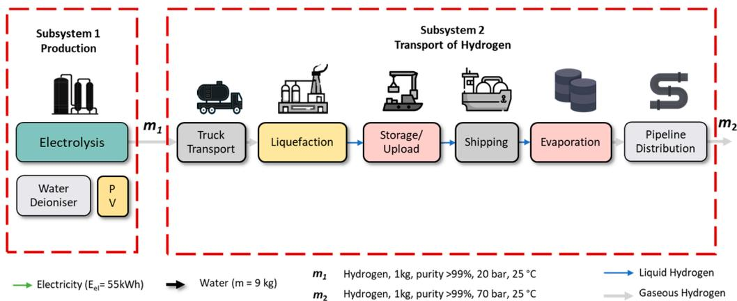
**Figure 3.** System boundary of the life cycle assessment. Icons copyright ©2023 Freepik Company S.L. [23].
