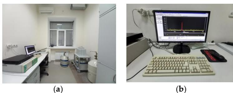
**Figure 3.** Gamma spectrometric setup: (a)—general view, (b)—spectrum displayed on a computer screen.
