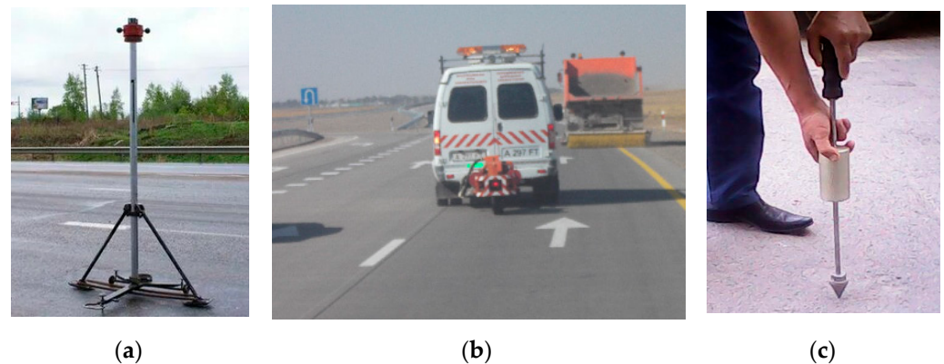
Figure 3. Instruments for measuring the friction coefficient—IkSp (a) and PKRS-2U (b)—and pavement surface hardness (c).
