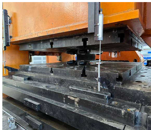
Figure 6. Experimental setup for compressive loading test of the rubber isolation bearing.
