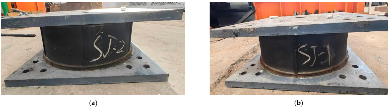
Figure 10. Post-test appearance of specimens after 200% shear strain under 8 MPa. (a) Traditional laminated rubber bearing. (b) Stiffness-reduced rubber isolation bearing.
