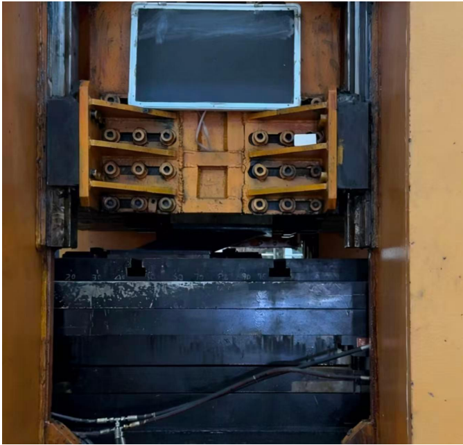
Figure 7. Experimental setup for the bearing under 100% shear deformation.
