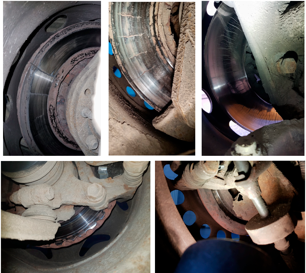
Figure 1. Examples of braking system component damage.
