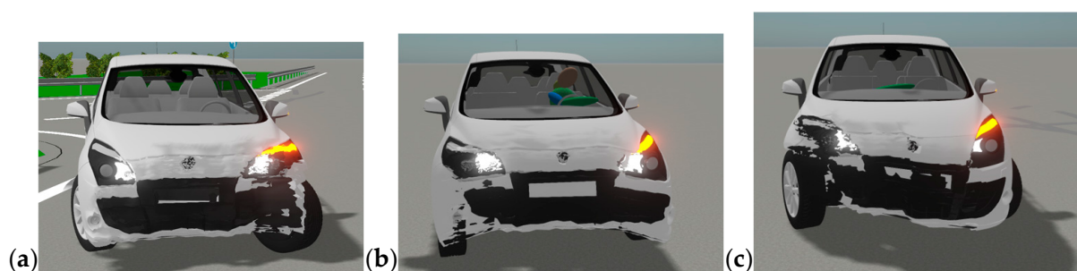
Figure 9. Damage to the car after collision with the truck: (a) truck speed—50 km/h, (b) 60 km/h, (c) 70 km/h.
