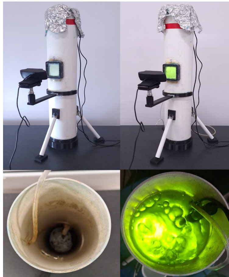
Figure 4. Smart bioreactor: (Left) inactive state, empty with no illumination; (Right) operational state, showing suspended Chlorella vulgaris and green LED lighting.
