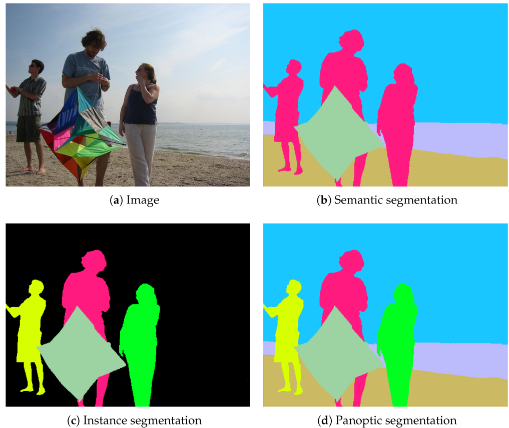
Figure 2. Example of semantic, instance, and panoptic image segmentation: (a) the original image; (b) semantic segmentation, with no distinction between each individual; (c) instance segmentation, distinguishing between individuals, but no segmentation of the background; and (d) panoptic segmentation, distinguishing between individuals while performing background segmentation. Reproduced from Jung et al. [24], licensed under CC BY 4.0.
