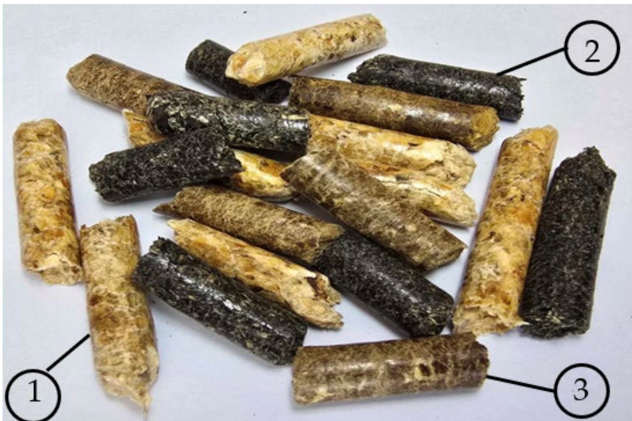
Figure 1. Studied samples: (1) wood pellets—W, (2) sunflower husk pellets—SH, (3) mixed blend pellets—W/SH.
