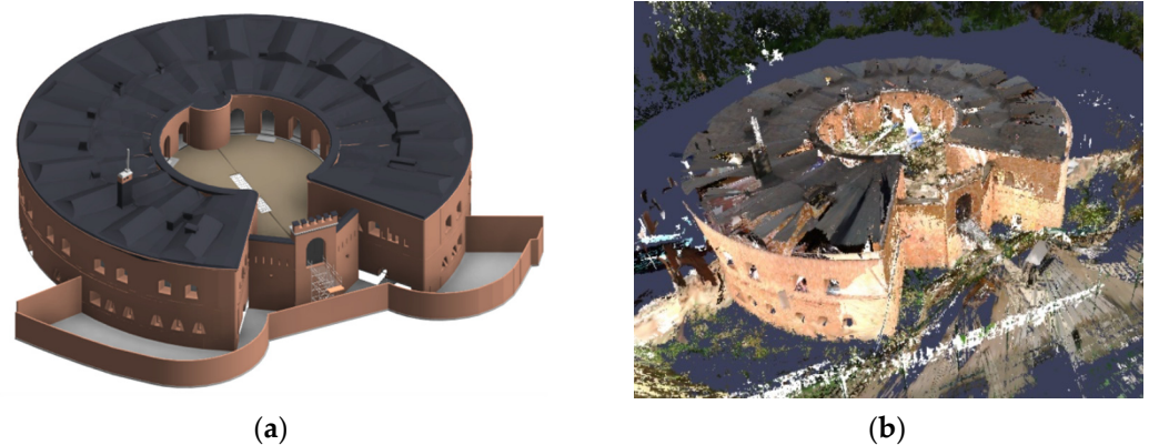
Figure 7. Fort renovation—BIM model (a) based on point cloud (b) (SXD Poland resources).
