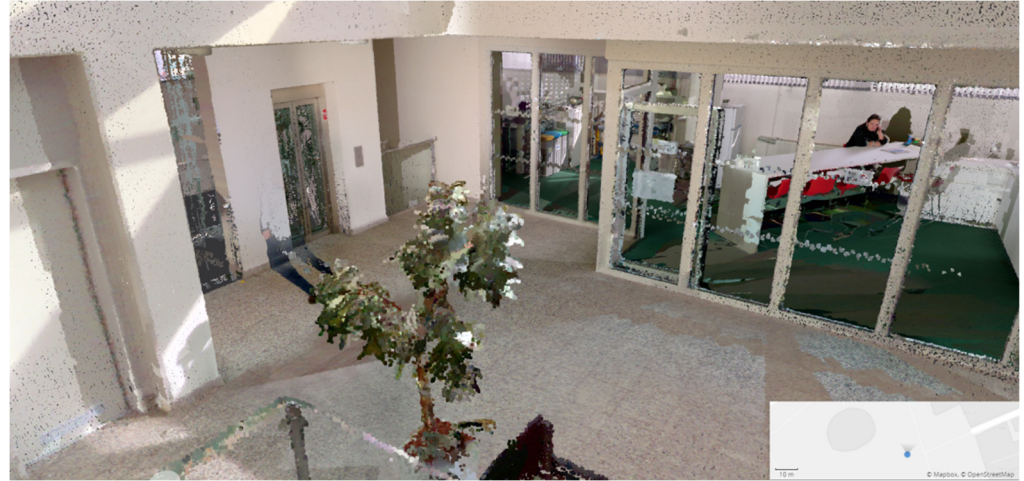
Figure 2. Example of a point cloud—office building—compiled with mobile scanner (SXD Poland (Warsaw, Poland) resource).
