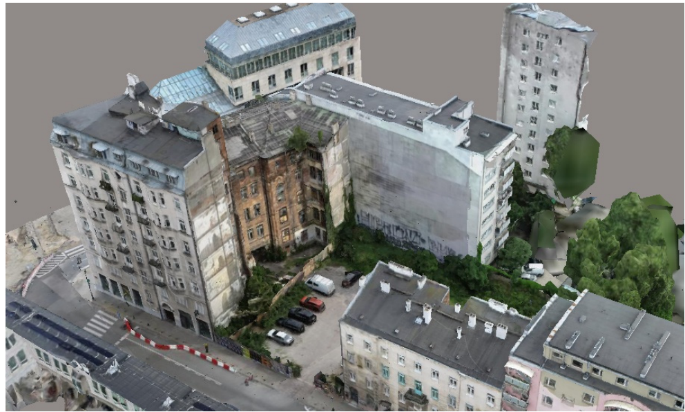
Figure 5. Three-dimensional mesh created with the use of digital photogrammetry (SXD Poland resource).
