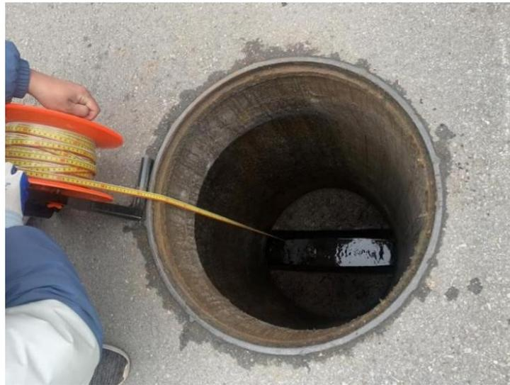
**Figure 9.** Actual depth of manhole cover node measured by water level meter.
