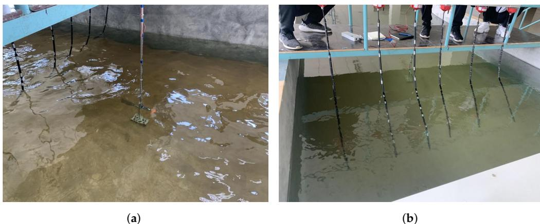
**Figure 8.** Experimental state of standard flow meter (a) and flexible smart water gauge (b).
