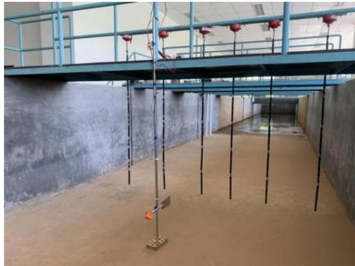
**Figure 7.** Experimental arrangement of terminal flexible water gauge and standard flow meter.
