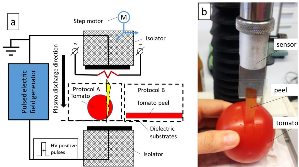
**Figure 2.** CAP treatment experimental scheme (a) and tomato peeling procedure based on texture analyzer system (b).
