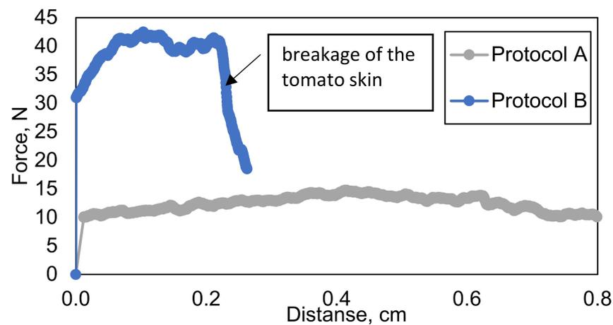
**Figure 4.** A specific peeling force graph of instrumental tomato peeling analysis for protocols A and B.
