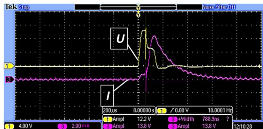
Figure 6. CAP treatment oscillogram of current and discharge.
