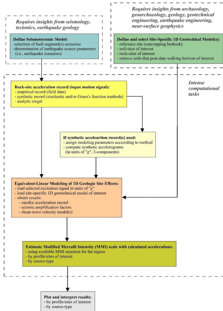
**Figure 4.** Schematized workflow of the proposed forward modeling of synthetic seismograms and 1D seismic site effects for an archaeoseismic project. The workflow honors an ancient earthquake's archaeological, geological and seismotectonic context. Modified with permission from [39]. Copyright 2016, Hinojosa-Prieto, H.R.
