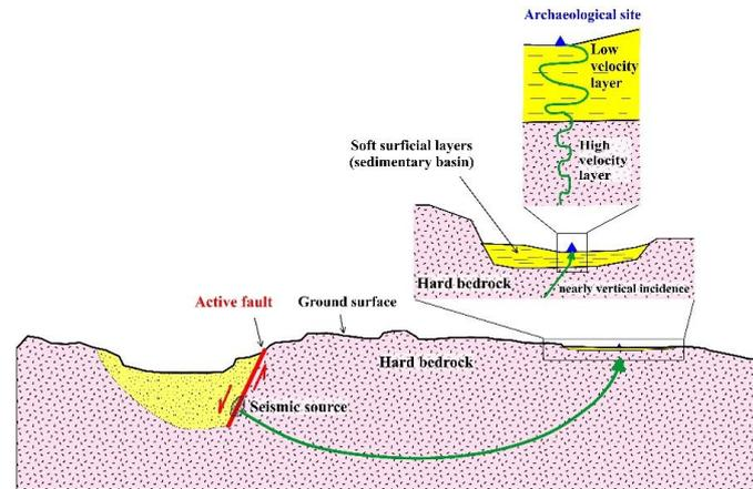
**Figure 1.** (Lower panel) Refraction processes that produce steep incidence of a seismic wave near the ground surface. (Middle and Upper panels) Zoomed areas where seismic wave amplification occurs due to the transition from higher velocity rock (higher impedance) to lower velocity sediments (lower impedance). Modified with permission from [18]. Copyright 2016, Hinojosa-Prieto, H.R.
