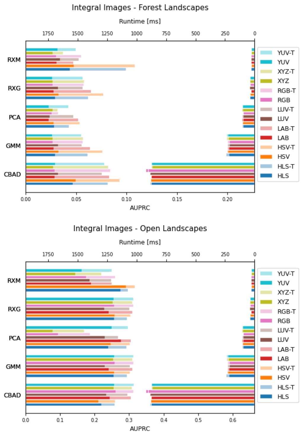
Figure 5. Performance in AUPRC (left bars) vs. runtime in ms (right bars): Color anomaly detection methods that produce results in less than a second. Reed–Xiaoli local (RXL) and local outlier factor (LOF) performed well but needed more than 20 seconds and are, therefore, not practicable for applications with real-time demands.
