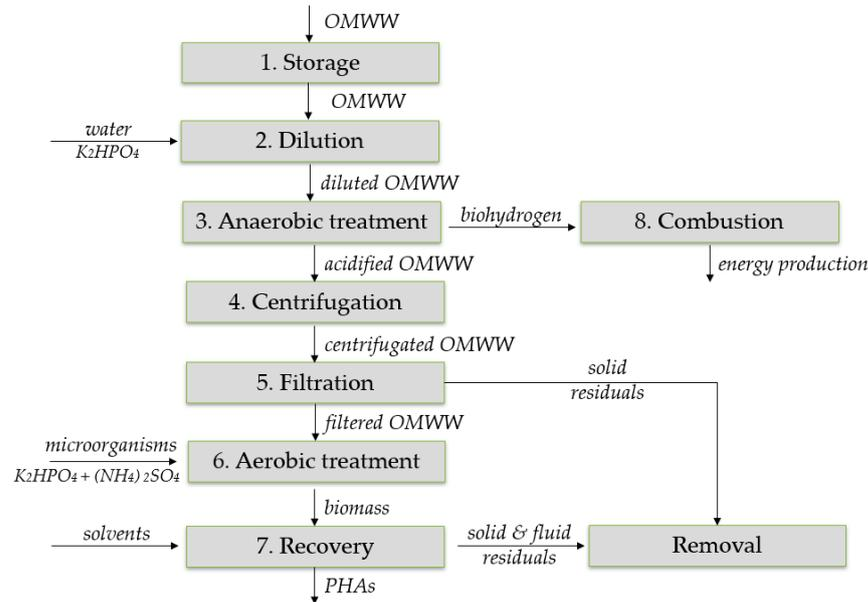
Figure 3. The 9 phases of the production process.
