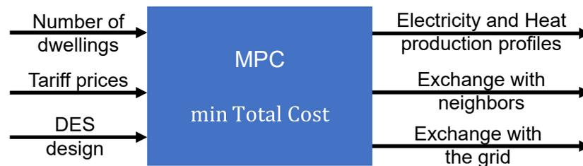
Figure 1. Inputs and outputs of the MPC optimization problem.
