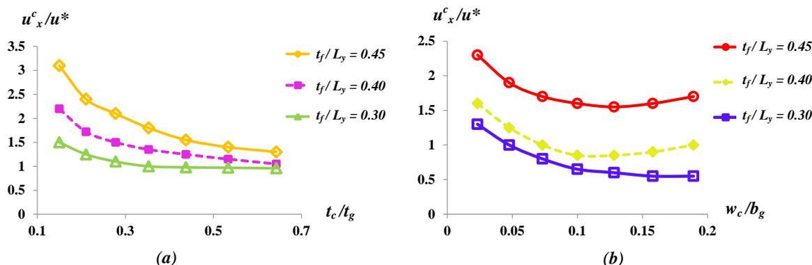
**Figure 6.** Variation of  $u_x^c/u^*$  as a function of (a)  $t_c/t_g$  in the range  $0.2 \leq t_c/t_g \leq 0.68$  and (b)  $w_c/b_g$  in the range  $0.03 \leq w_c/b_g \leq 0.2$  for different values of  $t_f/L_y$ .
