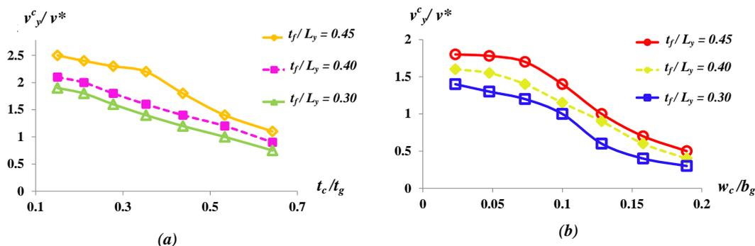
**Figure 7.** Variation of  $v_y^c/v^*$  as a function of (a)  $t_c/t_g$  in the range  $0.2 \leq t_c/t_g \leq 0.68$  and (b)  $w_c/b_g$  in the range  $0.03 \leq w_c/b_g \leq 0.2$  for different values of  $t_f/L_y$ .
