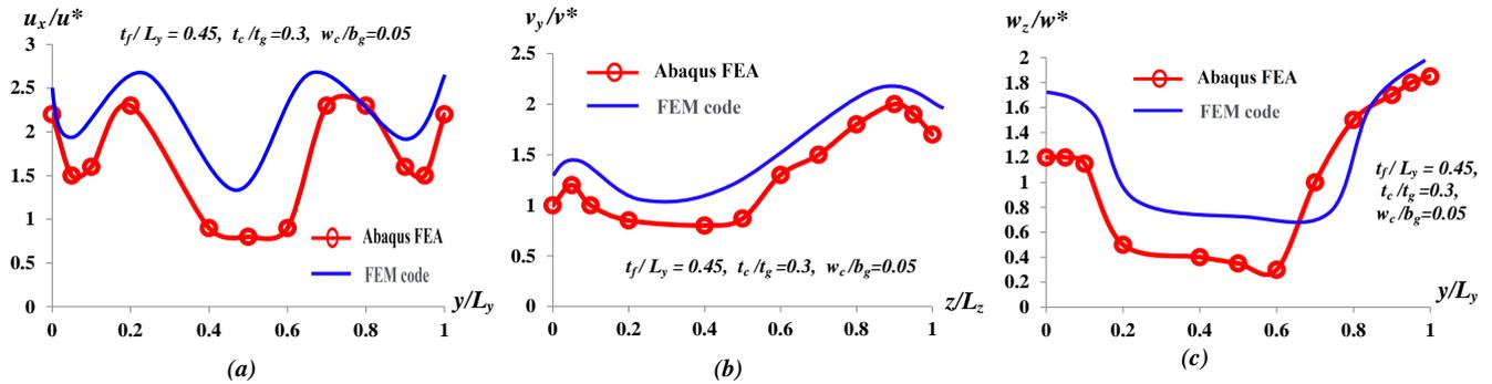
**Figure 4.** Distribution and comparison of different parts of displacement field between Abaqus FEA and FE model for (a)  $u_x/u^*$  along  $y$  at  $z = L_z/2$  for applied traction  $t_x$ ; (b)  $v_y/v^*$  along  $x$  at  $y = L_y/2$  for applied traction  $t_y$ ; (c)  $w_z/w^*$  along  $y$  at  $z = L_z/2$  for applied traction  $t_z$  at the tip of the blade (i.e.,  $x = L_x$ ) for  $t_f/L_y = 0.45$ ,  $t_c/t_g = 0.3$ , and  $w_c/b_g = 0.05$ .
