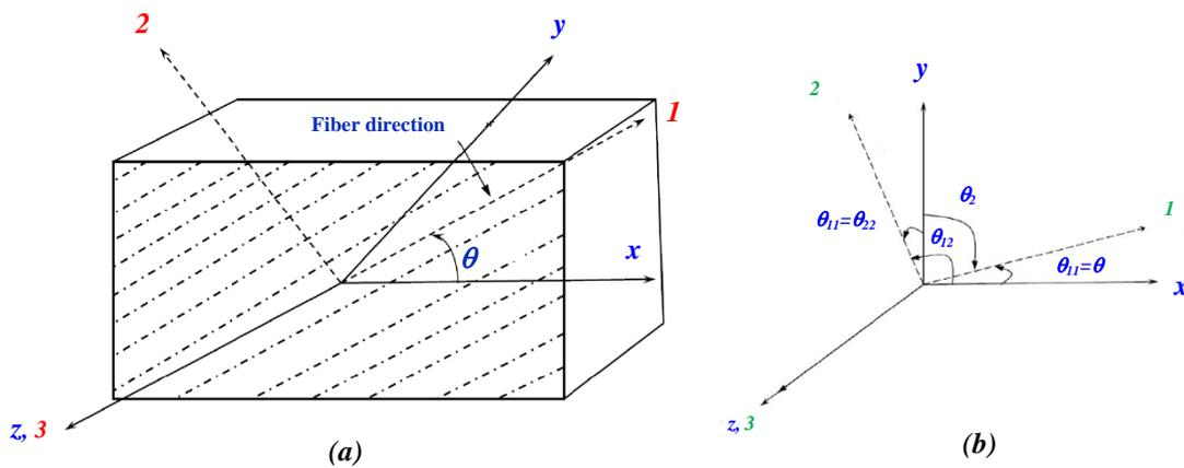
**Figure 1.** (a) Schematic of a unidirectional orthotropic composite laminate with principal material co-ordinate system (1, 2, and 3) and global co-ordinates ( $x, y,$  and  $z$ ). (b) Principal material axis 3 is rotated by  $\theta$  in  $x - y$  plane with anticlockwise angle with respect to  $x$ -axis is taken as positive.
