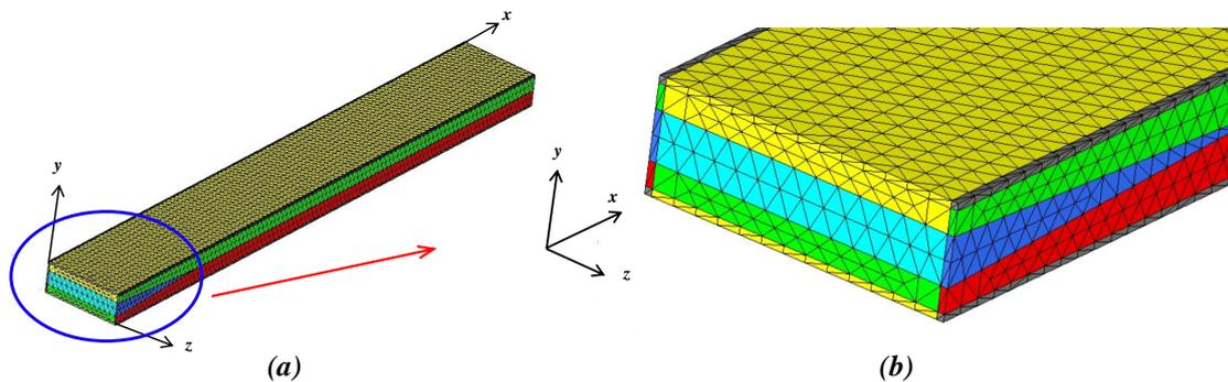
**Figure 3.** (a) Typical finite element mesh with linear tetrahedral elements in Hypermesh [37]; (b) zoomed part of the root showing the nodal continuity of different parts of composite laminate in the finite element (FE) model.
