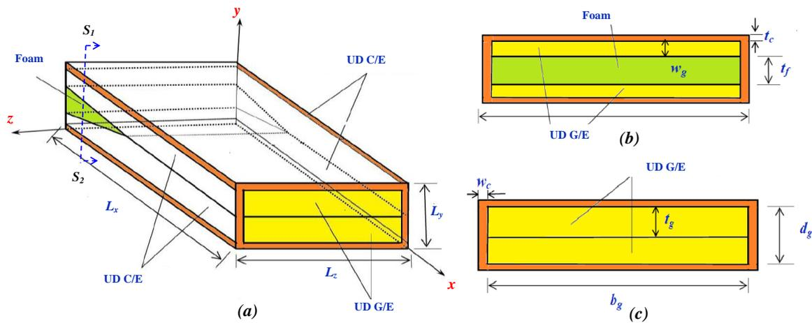
**Figure 2.** (a) 3-D beam geometry of the helicopter rotor blade consisting of unidirectional glass/epoxy (UD G/E), unidirectional  $\pm 45^\circ$  carbon/epoxy (UD C/E), and isotropic foam; (b) cross section near the root; (c) cross section at the tip of the rotor.
