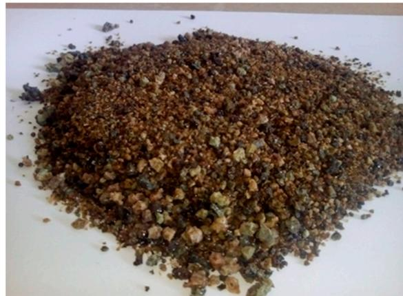
Figure 2. Water-cooled slag aggregate (WCS).
