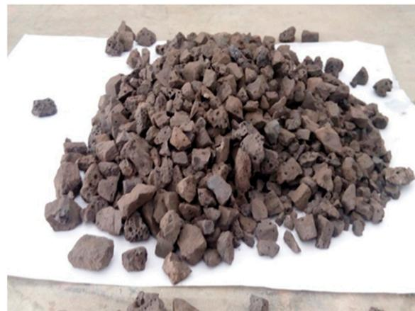
**Figure 1.** Air-cooled slag aggregate (ACS).
