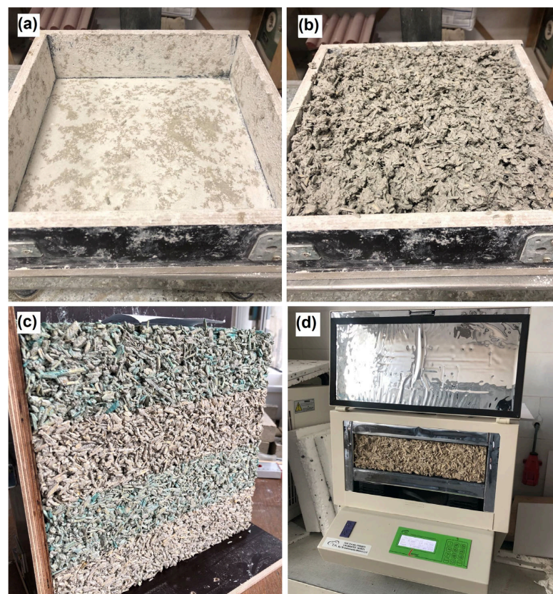
Figure 3. Key stages of specimen preparation and testing: (a) empty reference mould; (b) loose-fill material for \rho_L determination; (c) compacted specimen showing layered structure (dye visualization); and (d) thermal conductivity testing in FOX 314 apparatus.
