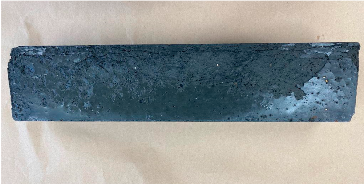
Figure 5. Photo of the 12 ksi steam-cured specimen after 330 cycles.
