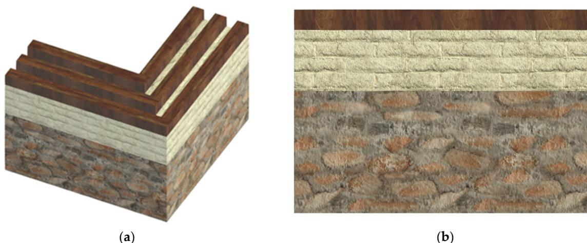
**Figure 2.** (a,b) Wooden ring beams spaced 0.60–1.00 m across the height of the masonry wall, designed in Revit.
