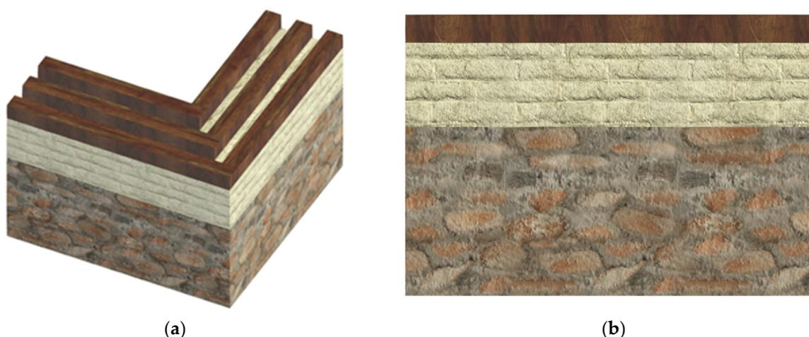
**Figure 2.** (a,b) Wooden ring beams spaced 0.60–1.00 m across the height of the masonry wall, designed in Revit.
