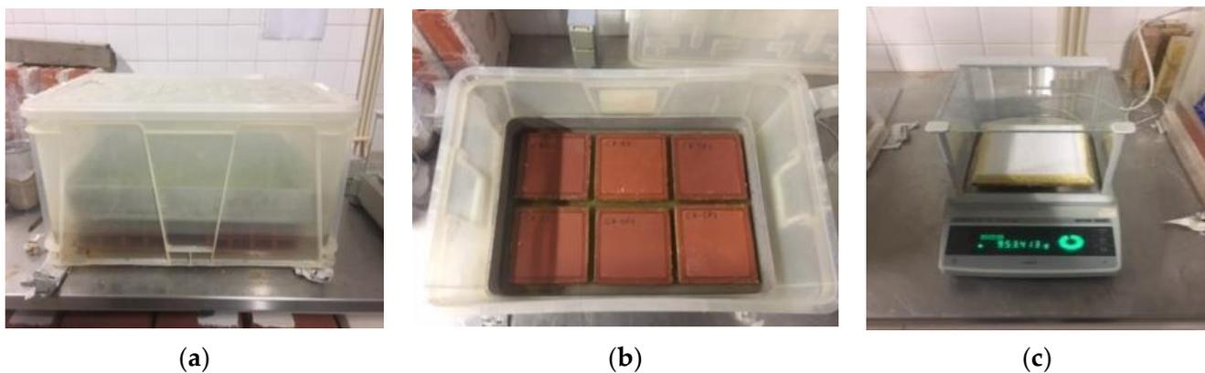
**Figure 7.** Water absorption test by capillarity: (a) test box; (b) placing the samples in the box with the painted base in contact with the water; (c) weighing of the samples.
