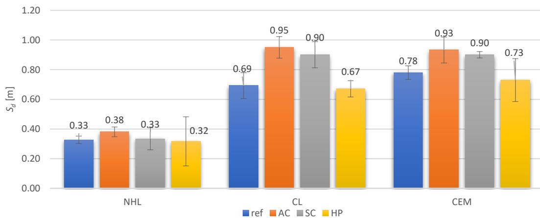
**Figure 16.** Diffusion equivalent air layer thickness values.
