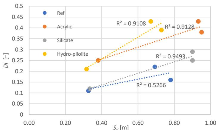
**Figure 17.** Correlation between the drying index ( $DI$ ) and the equivalent air layer thickness ( $S_d$ ).
