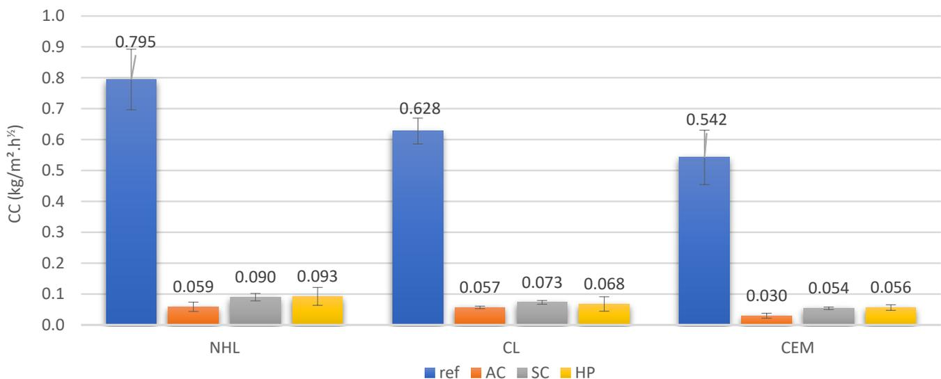
**Figure 8.** Coefficients of capillary water absorption.
