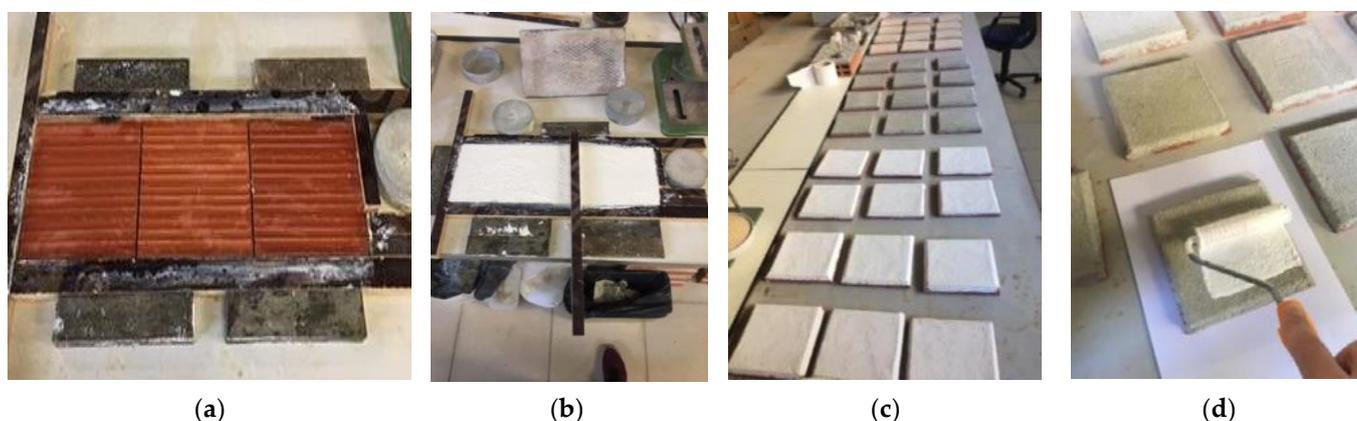
**Figure 2.** Stages of execution of the samples: (a) assembly of ceramic bases for the execution of samples; (b) application of hydrated lime render on the ceramic support; (c) samples in the drying process; (d) application of paint.
