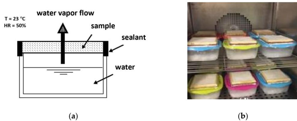
**Figure 15.** Water vapour permeability test: (a) schematic illustration of the capsule; (b) capsules inside the climatic chamber.
