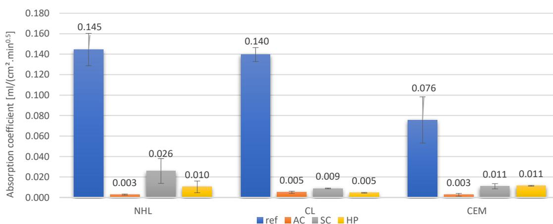
**Figure 14.** Low-pressure water absorption coefficient values.
