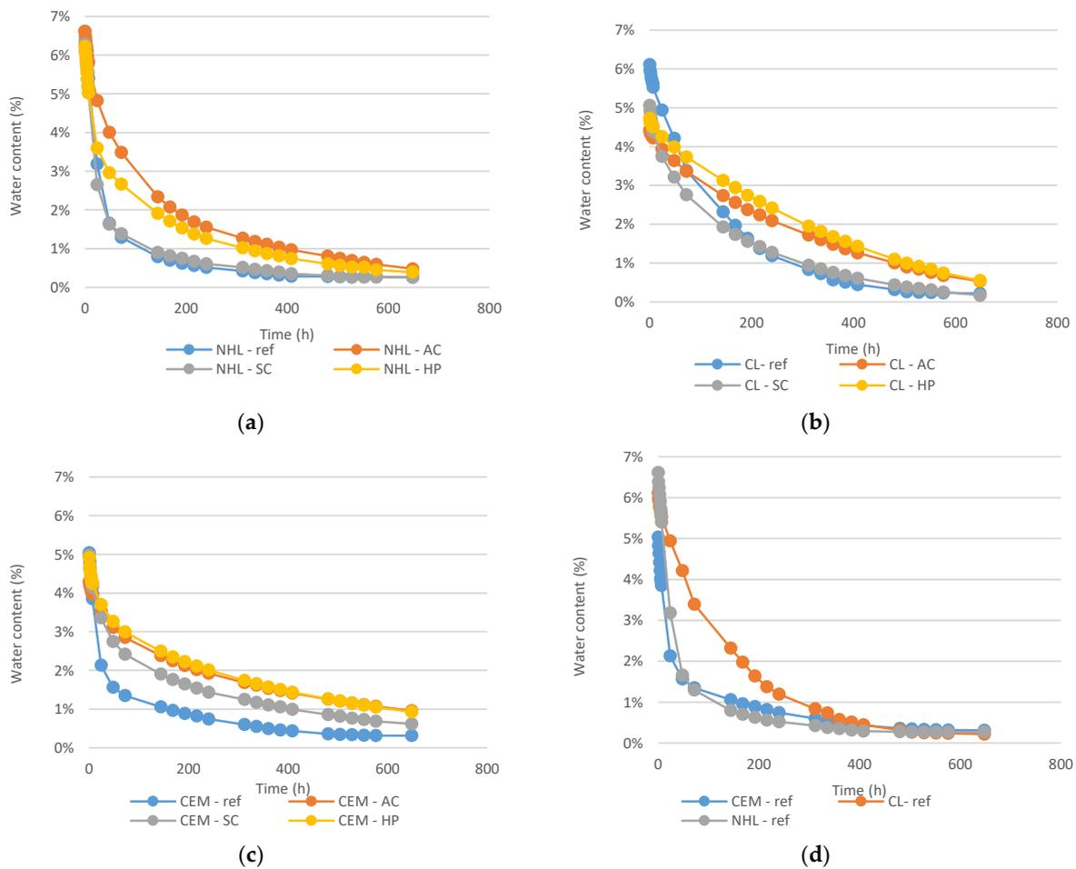
**Figure 10.** Drying curves resulting from the capillary test: (a) curves related to the NHL render; (b) curves related to CL render; (c) curves related to CEM render; (d) comparative curves of different renders without paint.
