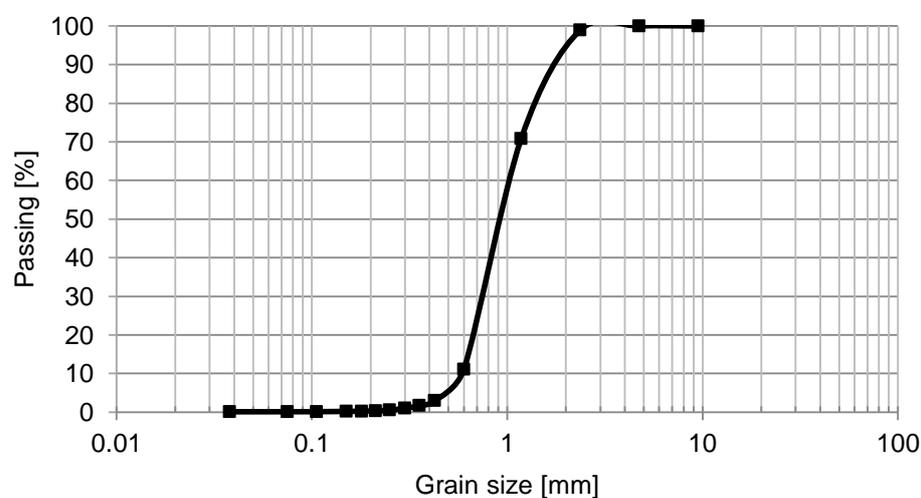
Figure 1. Aggregate particle size distribution curve.
