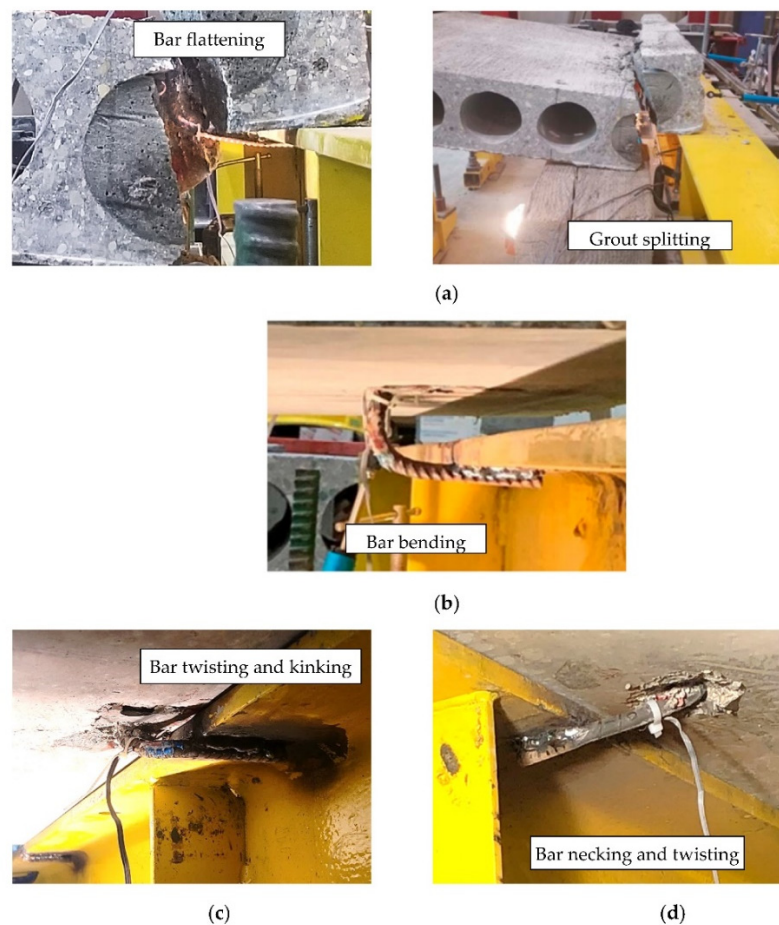
Figure 8. Mode of failure for side-bearing specimens: (a) SB-TN-90 (pulling/normal), (b) SB-CN-90 (pushing/normal), (c) SB-CP-90 (pushing/parallel), and (d) SB-TP-90 (pulling/parallel).
