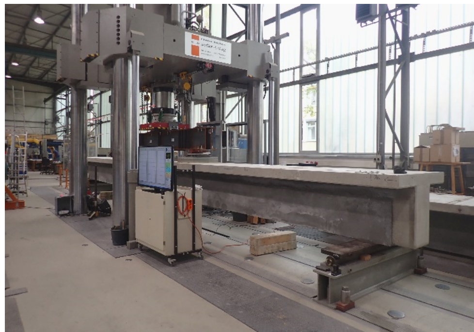
Figure 7. Large-scale component test during the individual approval process. (Photo: CARBOCON GMBH).
