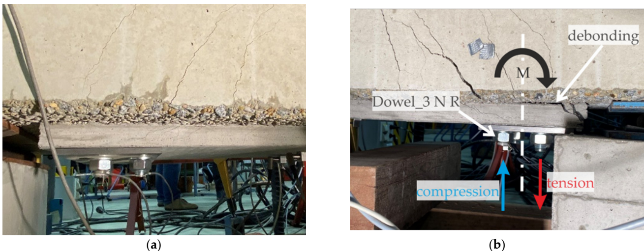
Figure 23. Anchored ends of the strengthening layer at the moment of failure of the right side: (a) left side; (b) right side. (Photos: CARBOCON GMBH).
