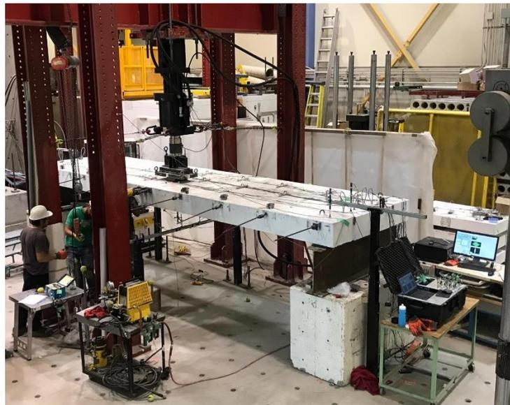
**Figure 3.** Load distribution test setup (vertical load applied at an interior girder).
