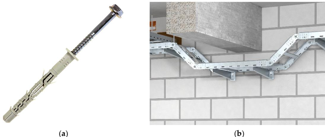
**Figure 5.** Example of a plastic anchor holding a fire rating for installations into concrete and masonry: (a) metal screw in plastic sleeve made of polyamide [34]. (b) Application example shows a cable tray fixed to a wall; the cables running on the tray to the fire control panel may be part of the active fire protection (courtesy OBO Bettermann).
