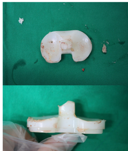
Figure 3. Removed polyethylene bearing with fracture on the upper-medial corner of the tibial post.
