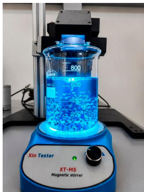
Figure 3. Scale-model prototype of water treatment using photocatalytic spheres under laboratory conditions.
