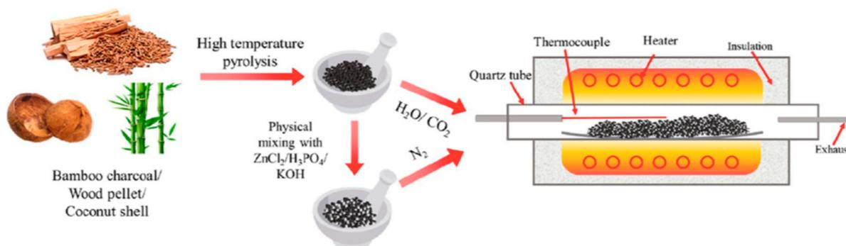
**Figure 2.** Schematic representation of biomass pyrolysis and biochar activation processes [15]. Copyright (2023) from the American Chemical Society.
