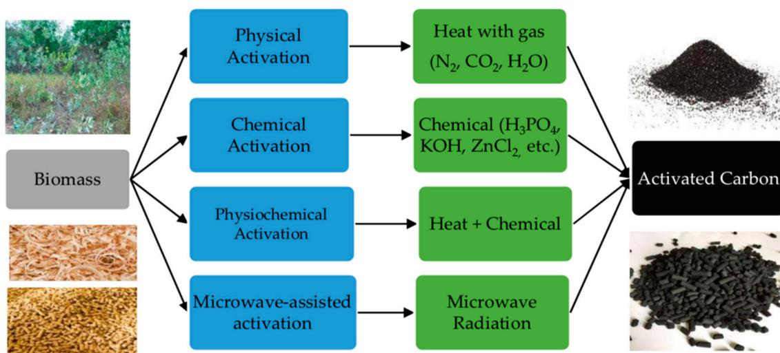
**Figure 10.** Technologies for activated carbon preparation from biomass. Adapted from reference [48].
