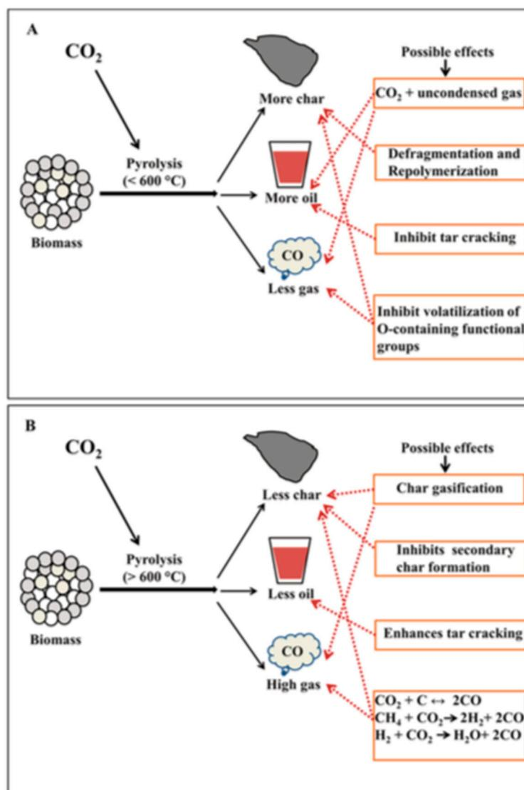
**Figure 13.** Possible effects of CO<sub>2</sub> on slow pyrolysis at (A) lower temperature range (300–600 °C) and (B) higher temperature range (600–800 °C). Adapted from reference [17].
