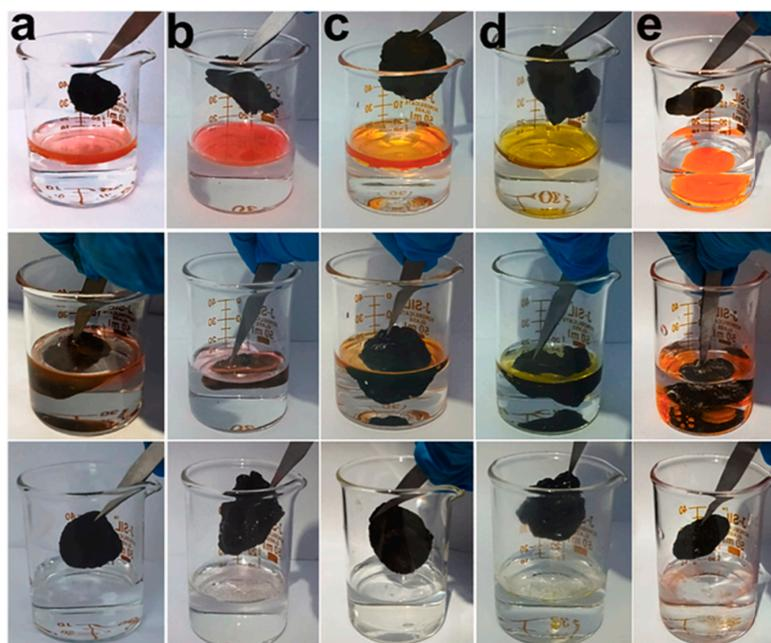
**Figure 9.** Cleanup of light and heavy oils ((a) silicon oil, (b) refined oil, (c) motor oil, (d) mustard oil, and (e) carbon tetrachloride) from an oil–water mixture by CD-coated cotton at room temperature. For better visualization, Nile red dye was added to the silicon oil, refined oil, and carbon tetrachloride [44]. Copyright (2022) Elsevier Ltd.
