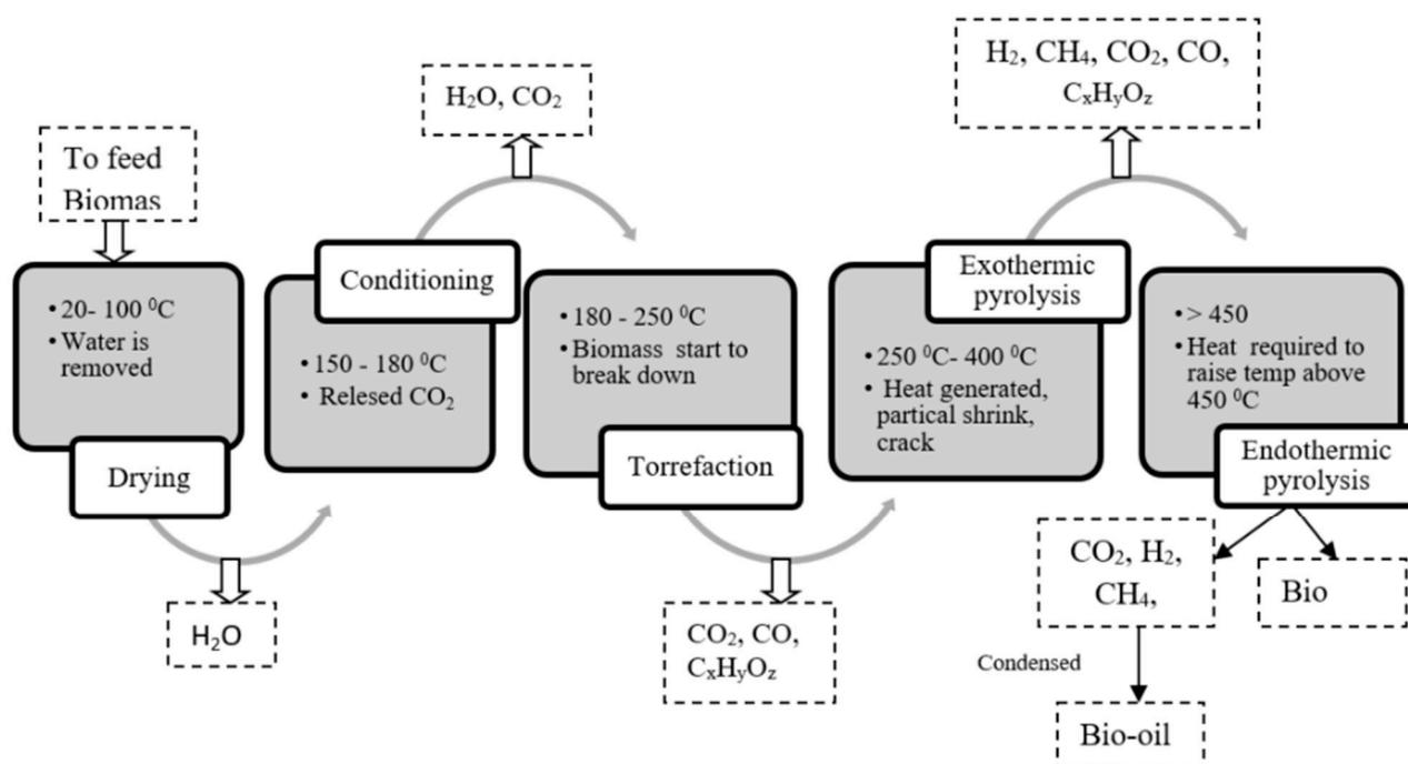
Figure 6. Biochar production process. Adapted from reference [31].
