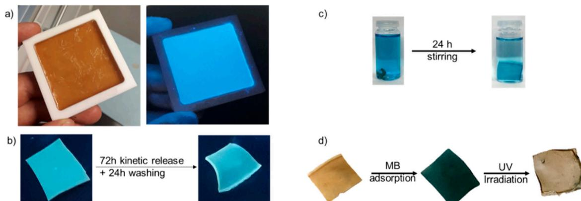
**Figure 8.** (a) PVA-CD hydrogel under visible light and UV light, (b) PVA-CD hydrogel fluorescence before and after washing treatment, (c) MB absorption test on PVA4 hydrogel, and (d) PVA4 hydrogel before and after MB adsorption and after 24 h of UV irradiation [43]. Copyright (2022) from the American Chemical Society.
