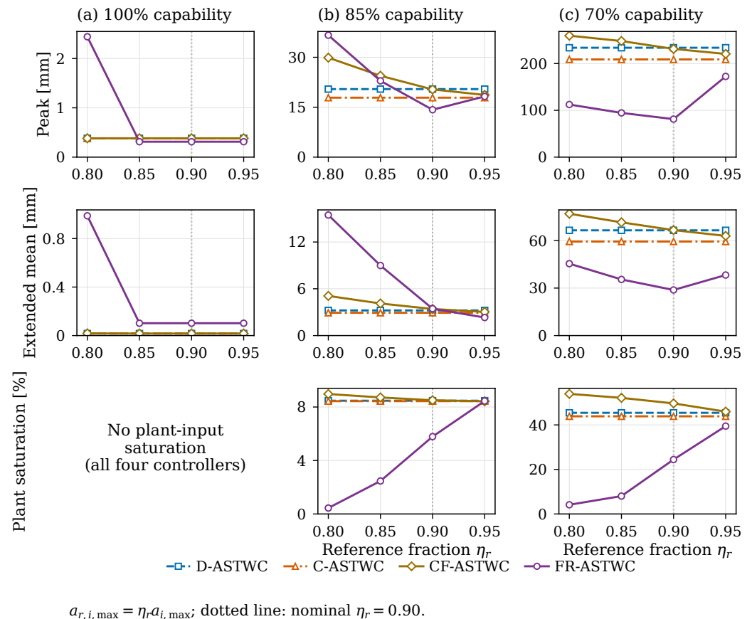
Figure 9. Sensitivity to the common CF/FR upstream-to-final acceleration limit ratio \eta_r = a_{r,i,\max}/a_{i,\max} . Only this ratio changes; all other parameters remain nominal. Peak and extended-window mean deformation are shown with plant saturation duty, exposing the trade-off between reference restriction and plant demand. These are deterministic local tests.
