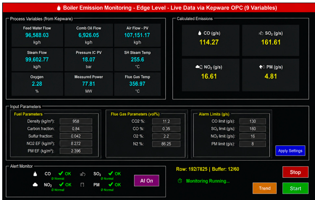
Figure 7. Edge-level real-time monitoring dashboard.
