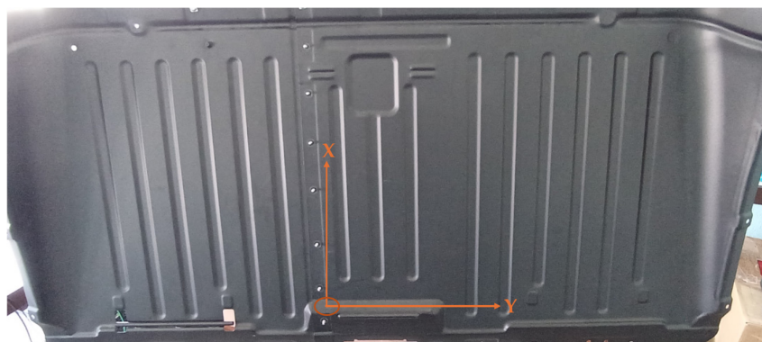
Figure 13. Reference defined on the Cloison plate.
