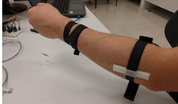
**Figure 2.** Optical fiber transducer attached to the forearm through Velcro straps.
