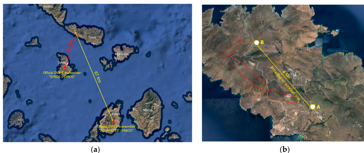
Figure 2. The interest point for DVB-T coverage; (a) The village of Pyrgos on Tinos island and the official DVB-T broadcast centers of Paros and Syros; (b) Area of Pyrgos village with the natural obstacles (mountains) that surround it, as well as indicative high points (A & B) where a 5 GHz link can be established. The red circles mark the mountains located in the surrounding area.
